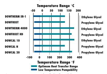
At appropriate concentrations, these fluids will provide burst protection to  ${\rm -100^{\circ}F}$  (-73  $^{\circ}{\rm C}$ ).
